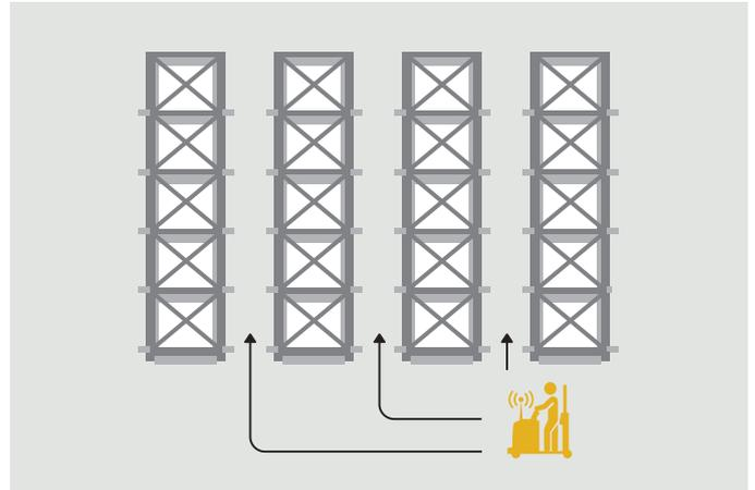
Stage 1 – Engineer manually moves the robot around the warehouse.
