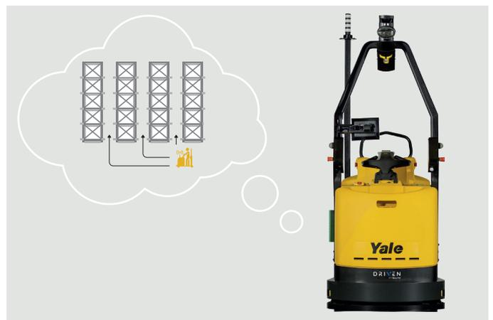
Stage 3 – Reference map is integrated into the robot's computer.
