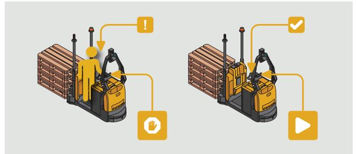
By switching from automatic mode to manual mode at the touch of a button, or movement of the tiller, the robotic lift truck can easily accommodate changing operational needs, giving the operator the opportunity to take control when appropriate and perform other tasks as and when required.
