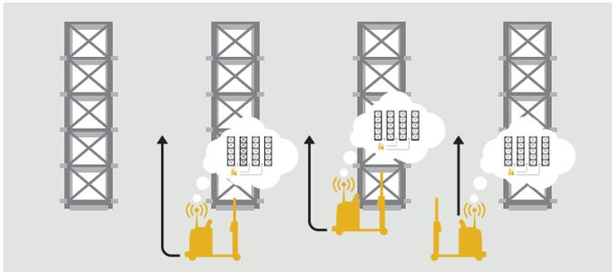
The geoguidance navigation technology works without the need for dedicated infrastructure, enabling it to integrate easily into existing operations. It simply maps the physical features and structures to self-locate and navigate, which means it's quick and easy to modify or create entirely new paths when there are changes to the environment, or to the missions that your robots are required to complete.
