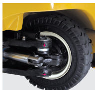
Extended steering axle for class leading manoeuvrability
