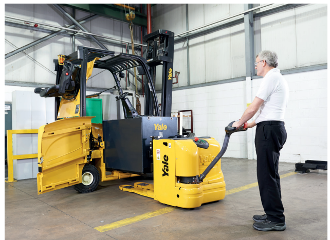
MS HBE powered battery side extractor
